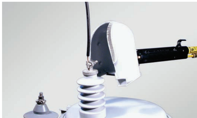
3. Place the guard onto the target bushing, taking care to position the trigger between the top and second bushing sheds.
