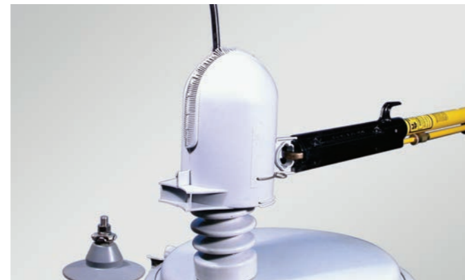
4. As the trigger makes initial contact with the bushing, it collapses, closing the guard around the bushing and leads. Disengage the shotgun stick from the guard handle and withdraw it. Installation is complete.
