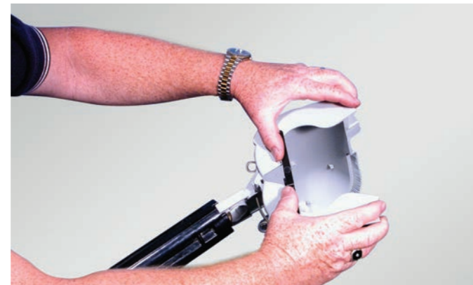
2. Cock open the guard using the integral trigger. Note: Triggered installation is optional for level, straight-on shotgun stick applications. The taper on the leading edge of the guard allows the guard to be easily installed by pushing it, uncocked, against the top bushing shed.
