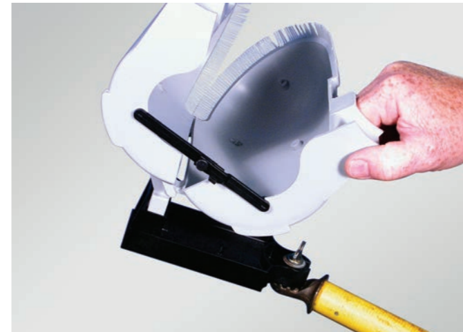
3. Insert the handle of the cocked guard into the adapter pocket.
